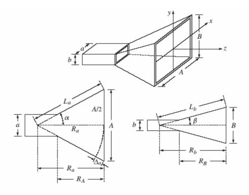
Considering the geometry depicted in figures the the various lengths and flare angles are given by:
