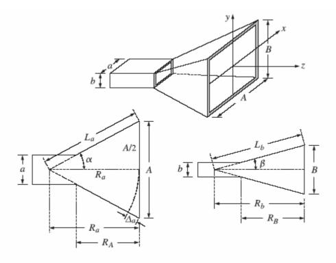
It follows from the geometry that the various lengths and flare angles are given by:
